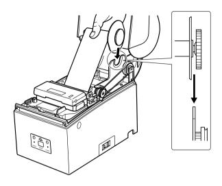
17) Turn the rewinder shaft clockwise to take up the slack in the paper.
