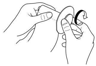
11) Grasp the center of the paper with your fingers to keep it from coming off of the rewinder and then set the rewinder shaft in the frame for the rewinder.
