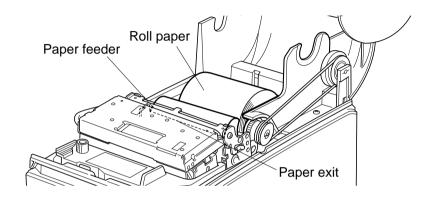
7) After the automatic paper feed has been completed, the POWER lamp (green) on the operating panel will blink.
