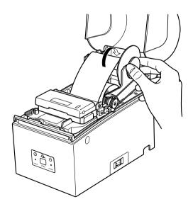
18) Close the cover and press the FEED button one time. Becomes a allowable print and complete the setting.
