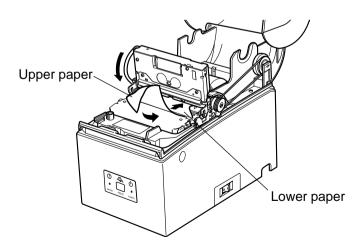
13) Pass the leading edge of the paper through the slit in the rewinder shaft until it extends 3 to 4 centimeters beyond it.
