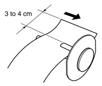
14) Fold the paper back so that it is held in place by the slit.
