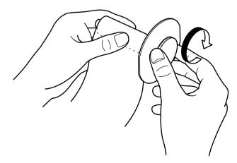
16) Grasp the center of the paper with your fingers to keep it from coming off of the rewinder and then set the rewinder shaft in the frame for the rewinder.
