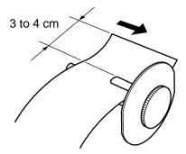
9) Fold the paper back so that it is held in place by the slit.
