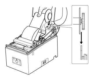
12) Turn the rewinder shaft clockwise to take up the slack in the paper.
