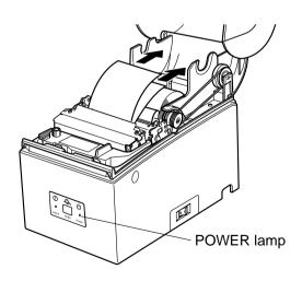
8) Pass the leading edge of the paper through the slit in the rewinder shaft until it extends 3 to 4 centimeters beyond it.
