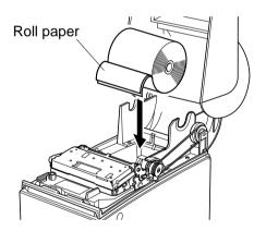
5) Insert the edge of the paper into the paper feeder (black plastic part). If inserted correctly, the edge of the paper will pass through the auto cutter paper slit.
